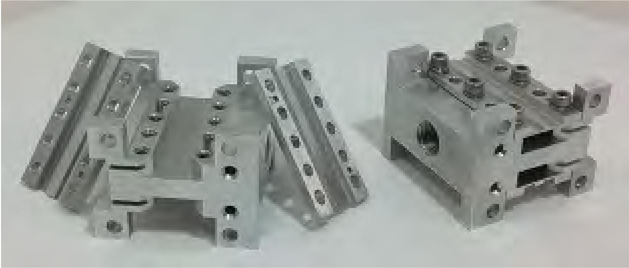
Dual Waveguide Housings
